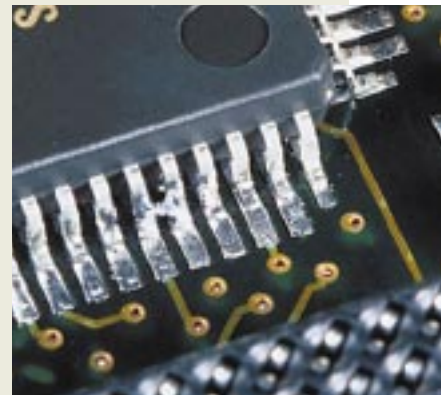
Teradyne’s automated-optical-inspection system (left) employs multiple cameras and light sources to unambiguously resolve tombstoned components (center) and solder bridges (right) in a high-speed production environment.
